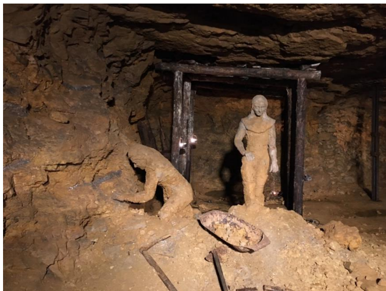
Figure 4. A typical excavation in the Frederic Pb-Ag ore mine in Tarnowskie Góry. Ore-bearing dolomite and galena veins are visible on the sides.
